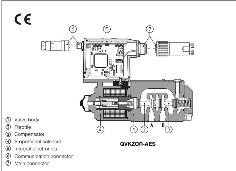
QVHZO and QVKZOR are 2 or 3 flow proportional valves, direct operated without position transducer, which provide compensated flow control according to the electronic reference signal.
