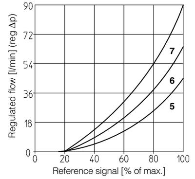
**13.2 Regulated flow/outlet pressure diagrams**
